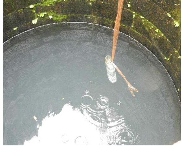
Taking sample with sterilised whiskey bottle at drinking water well 1
