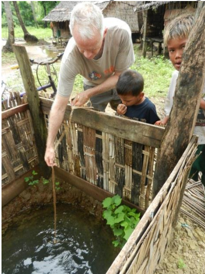
Sample at unlined earthen wall washing well
